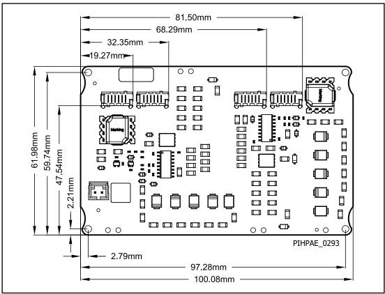
Figure 5. Top View of 2SML0220D2E0(C).
