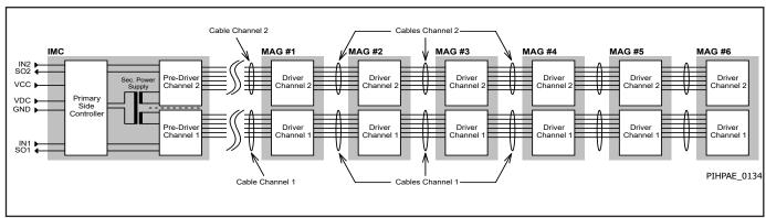
Figure 3. Functional Block Diagram of 2SIL1200T2A0(C) with 6 2SML0220D2E0(C) MAGS
