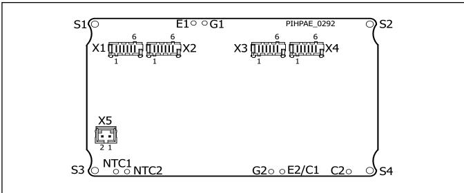
Figure 2. Pin Configuration of 2SML0220D2E0(C).
