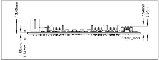
Figure 6. Side View of 2SML0220D2E0(C).
