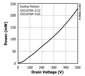
Figure 16. Drain Capacitance Power.
