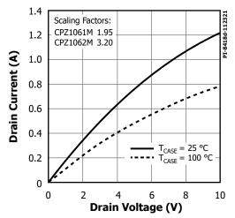
Figure 10. Output Characteristics.
