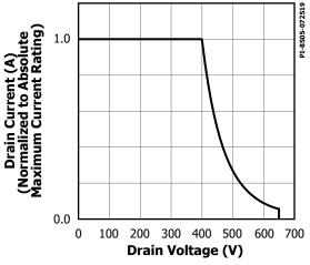
Figure 9. Maximum Allowable Drain Current vs. Drain Voltage.
