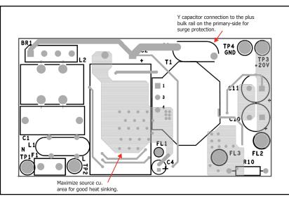
Figure 6. PCB Layout Top Side.
