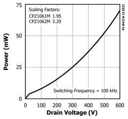
Figure 12. Drain Capacitance Power.
