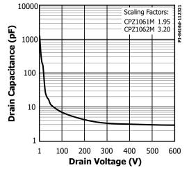
Figure 11.  $C_{oss}$  vs. Drain Voltage.
