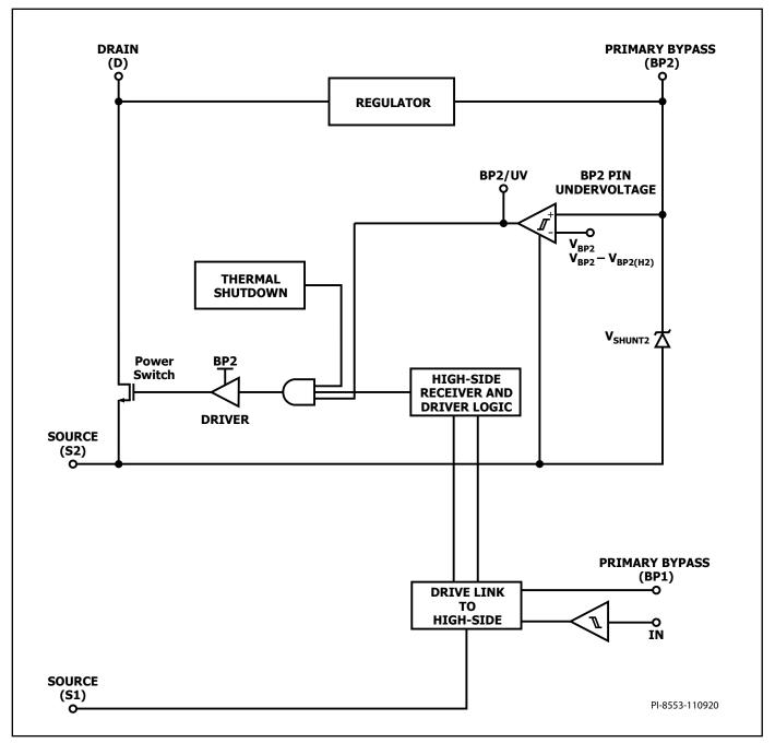
Figure 3. Block Diagram.
