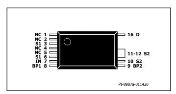
Figure 4. Pin Configuration.
