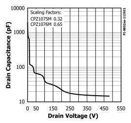
Figure 15. C<sub>oss</sub> vs. Drain Voltage.
