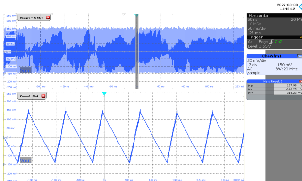
Figure 52 – Output Ripple, LL Burst (0.4 A), 115 VAC. Blue: V_{OUT} , 50 mV / div. Ripple: 1.31% Ripple.
