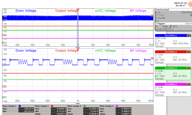
Figure 96 – uVcc Normal Operation Waveforms. 85 VAC, 5 Vo Load 1 A. Drain Voltage: 200 V / div., 2 ms / div. Output Voltage: 2 V / div., 2 ms / div. uVCC Voltage: 1 V / div., 2 ms / div. BP Voltage: 2 V / div., 2 ms / div. uVCC max = 3.3281 V
