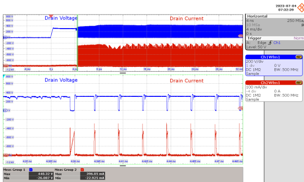
Figure 36 – Drain Voltage and Current Waveforms. 85 VAC, 1 A Output. Drain Voltage: 100 V / div., 4 ms / div. Drain Current: 100 mA /div., 4 ms / div. Zoom = 15 \mu s / div. I_{DS(MAX)} = 328.85 mA, V_{DS(MAX)} = 243.87 V.
