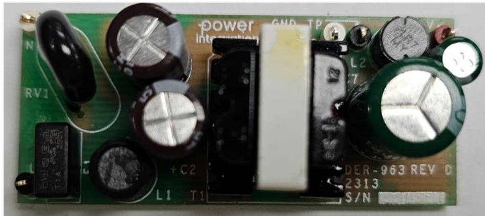
Figure 1 – Populated Circuit Board Photograph, Top.
