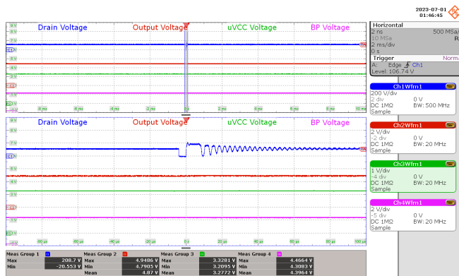
Figure 96 – uVcc Normal Operation Waveforms. 85 VAC, 5 Vo Load 1 A. Drain Voltage: 200 V / div., 2 ms / div. Output Voltage: 2 V / div., 2 ms / div. uVCC Voltage: 1 V / div., 2 ms / div. BP Voltage: 2 V / div., 2 ms / div. uVCC max = 3.3281 V
