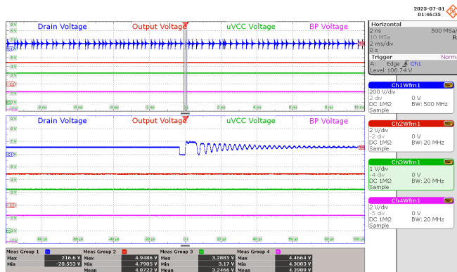
Figure 100 – uVcc Normal Operation Waveforms. 85 VAC, 5 Vo Load 1 A. Drain Voltage: 200 V / div., 2 ms / div. Output Voltage: 2 V / div., 2 ms / div. uVCC Voltage: 1 V / div., 2 ms / div. BP Voltage: 2 V / div., 2 ms / div. uVCC max = 3.2885 V
