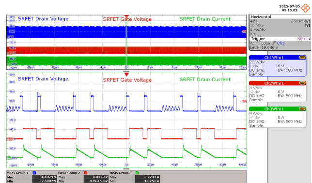
Figure 49 – SR FET Waveforms. 115 VAC, 1 A Output. SR FET Drain Voltage: 10 V / div., 4 ms / div. SR FET Gate Voltage: 4 V / div., 4 ms / div. SR FET Drain Current: 4 A / div, 4 ms / div. Zoom: 20 μs / div. SR FET V DS(MAX) : 23.992 V.
