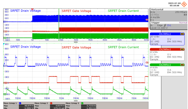
Figure 59 – SR FET Waveforms. 265 VAC, 1 A Output. SR FET Drain Voltage: 20 V / div., 4 ms / div. SR FET Gate Voltage: 4 V / div., 4 ms / div. SR FET Drain Current: 4 A / div., 4 ms / div. Zoom: 20 \mu s / div. SR FET V_{DS(MAX)} : 40.079 V.
