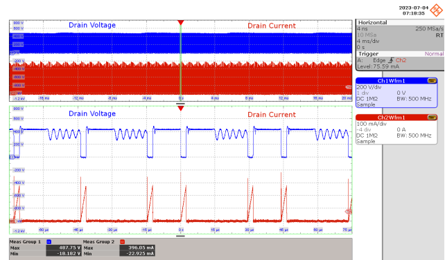
Figure 29 – Drain Voltage and Current Waveforms. 115 VAC, 1 A Output. Drain Voltage: 100 V / div., 4 ms / div. Drain Current: 100 mA /div., 4 ms / div. Zoom = 15 \mu s / div. I_{DS(MAX)} = 340.71 mA, V_{DS(MAX)} = 283.4 V.
