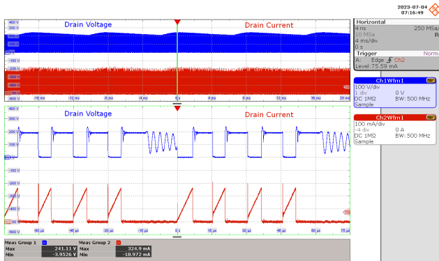
Figure 28 – Drain Voltage and Current Waveforms. 85 VAC, 1 A Output. Drain Voltage: 100 V / div., 4 ms / div. Drain Current: 100 mA /div., 4 ms / div. Zoom = 15 \mu s / div. I_{DS(MAX)} = 324.9 mA, V_{DS(MAX)} = 241.11 V.
