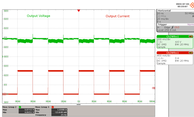
Figure 132 – Transient Output Waveforms. 85 VAC. Output Voltage: 200 mV / div., 20 ms / div. Output Current: 400 mA / div., 20 ms / div. Load Transient: 0 % - 100%. Duty Cycle, Slew Rate: 50%, 0.8 A / \mu s. Frequency: 25 Hz. V_{MAX} : 5.0743 V, V_{MIN} : 4.8451 V.
