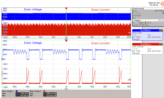
Figure 28 – Drain Voltage and Current Waveforms. 85 VAC, 1 A Output. Drain Voltage: 100 V / div., 4 ms / div. Drain Current: 100 mA /div., 4 ms / div. Zoom = 15 \mu s / div. I_{DS(MAX)} = 324.9 mA, V_{DS(MAX)} = 241.11 V.
