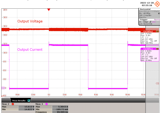
Figure 105 – 100 VAC 60 Hz, 0-5 A Transient Load. CH2(Red): V_{OUT} , 2 V / div., 2 ms / div. CH3(Pink): I_{OUT} , 1 A / div. V_{OUT(MAX)} = 15.61\text{ V} , V_{OUT(MIN)} = 14.82\text{ V} .
