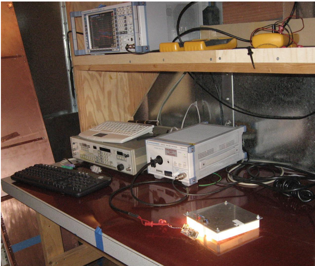
Figure 48 – Conducted Emissions Measurement Set-up.
