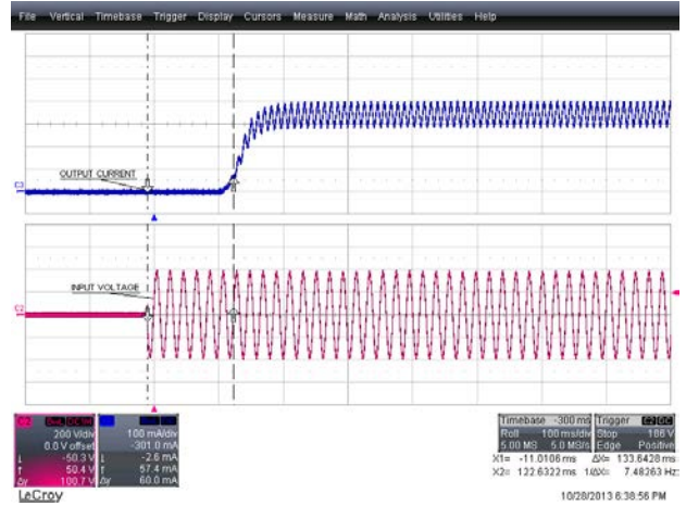
Figure 32 – 265 VAC, 50 Hz. Upper: I_{OUT} , 100 mA / div. Lower: V_{IN} , 200 V, 100 ms / div. Start-up Time: 133 ms
