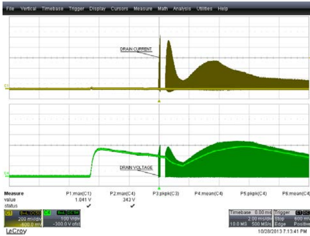
Figure 39 – 195 VAC, 50 Hz Start-up. Upper: I_{DRAIN} , 200 mA / div. Lower: V_{DRAIN} , 100 V, 2 ms / div.
