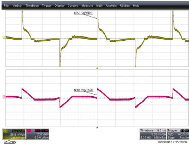
Figure 61 – 60° Conduction Angle. Upper: I_{IN} , 50 mA / div. Lower: V_{IN} , 200 V, 5 ms / div.
