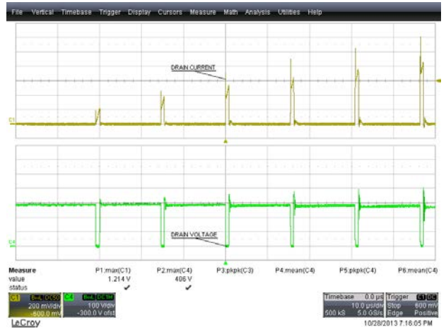
Figure 42 – 265 VAC, 50 Hz Start-up. Upper: I_{DRAIN} , 200 mA / div. Lower: V_{DRAIN} , 100 V, 10 \mu s / div.
