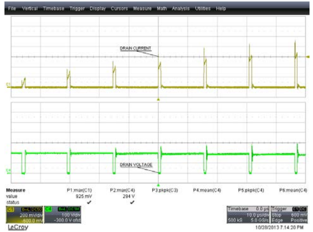
Figure 40 – 195 VAC, 50 Hz Start-up. Upper: I_{DRAIN} , 200 mA / div. Lower: V_{DRAIN} , 100 V, 10 \mu s / div.
