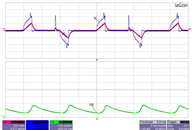
Figure 84 – 240 VAC / 50 Hz, (Germany) Busch 691 U-101 Dimmer at Minimum TRIAC Conduction. Load: 36 V LED String. Ch2: V_{IN} , 200 V / div. Ch3: I_{IN} , 100 mA / div. Ch4: I_{OUT} , 100 mA / div. Time Scale: 5 ms / div.
