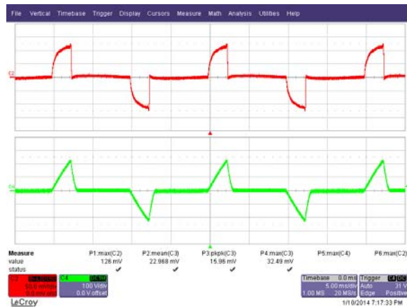
Figure 57 – 43°Conduction Angle. Upper: I_{IN} , 50mA / div. Lower: V_{IN} , 100 V, 5 ms / div.
